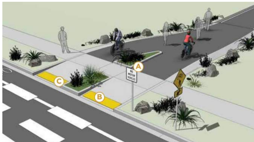
Figure 13: Bollard Alternatives, 2017 Empire State Trail Design Guide, page 5-34
